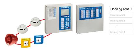
The modular Extinguishing Control Panels LC600 can be expanded to up to 128 flooding zones which can be assigned to a maximum of 128 extinguishing systems. Every sectional control panel of a networked Control Panel BCnet600 can be upgraded to up to 128 flooding zones. The total number of flooding zones that are managed and can be operated in the security network is limited to 2048 flooding zones.
